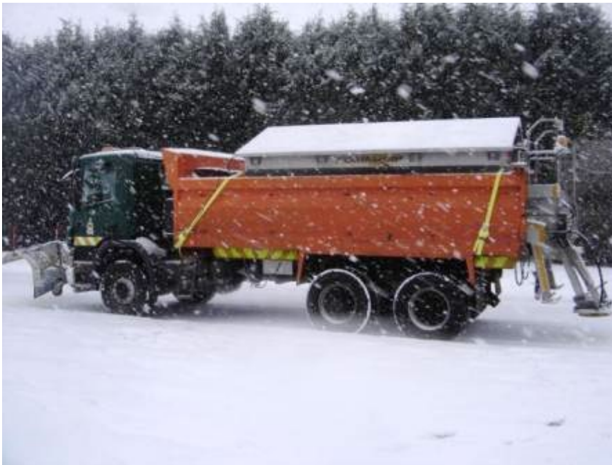
Figure 4: Demountable salt spreader
