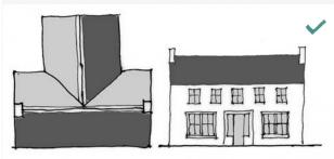
ALTERNATIVE TOR L'SHAPED PLAN NOTE: REDUCED ROOF VOLUME .
