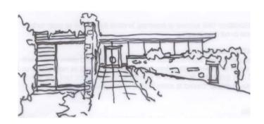
A low flat roofed house, if carefully designed, and finished using natural materials such as wood and stone, will have a very low visual impact on the landscape and may allow for a more prominent setting. Note a vegetation planted roof finish would be possible here, this would have an insulating effect.
